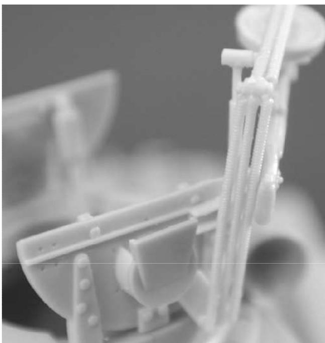
Then glue the pin on the left side of the suspension arm to the hole on the right side of the vertical support tube cast onto the new hatch as shown.
